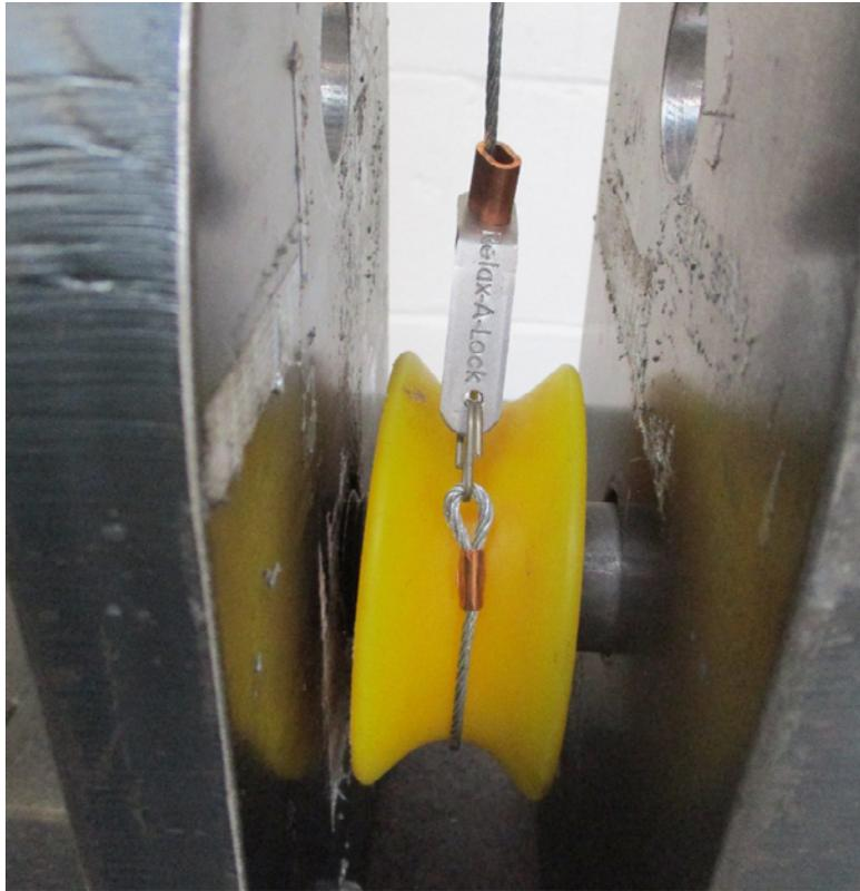
Figure 3.3: Snare loop on plastic spool mounted in clevis arrangement.
