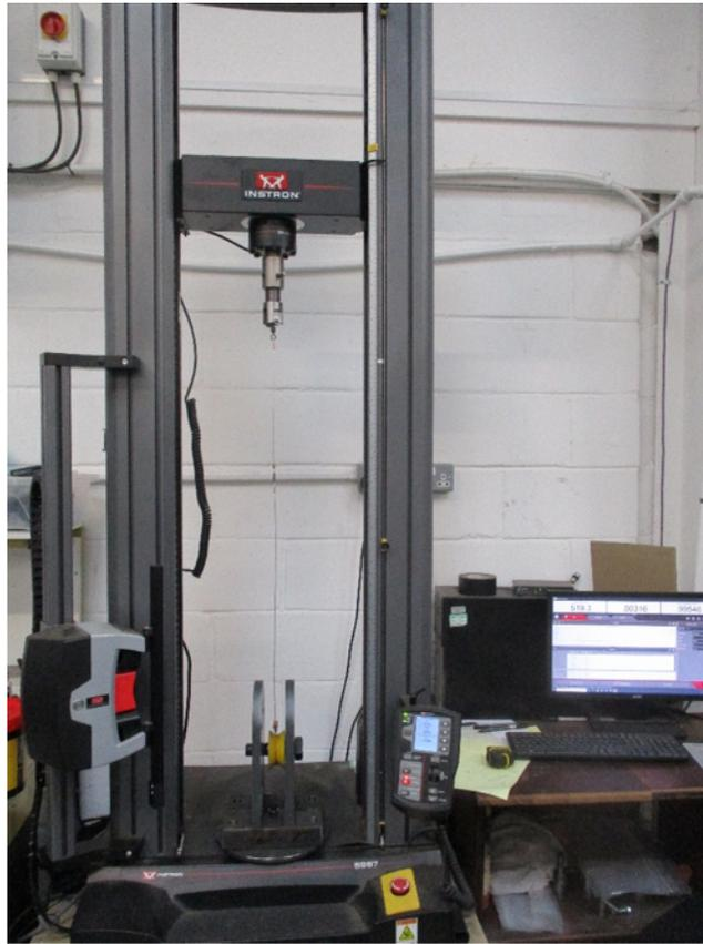
**Figure 3.1:** INSTRON tensile testing machine with DB snare mounted ready for testing.
