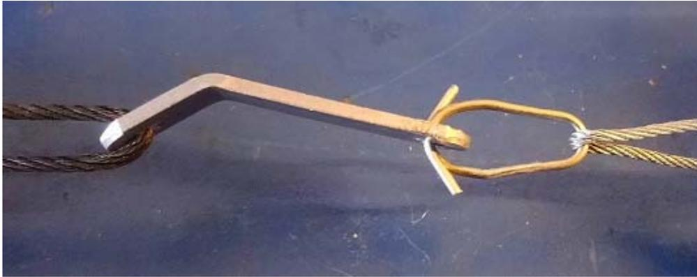
**Figure 6.1:** Configuration employed in the tests to measure the breaking strength of the breakaway clip undertaken for Perdix (from [4]).
