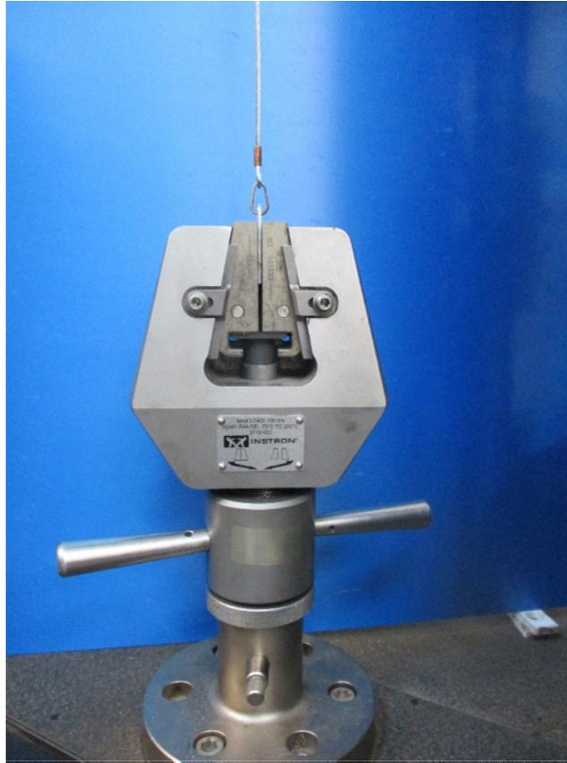
**Figure 6.4:** Measuring the strength of the breakaway clip in the straight configuration.
