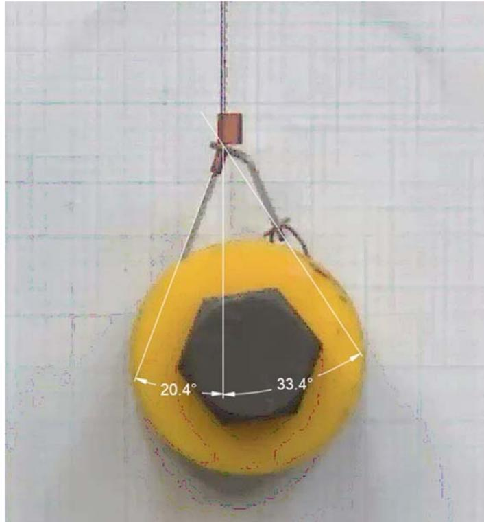
**Figure 6.3:** Photograph showing the geometry of the snare over the spool when under a vertical load of approximately 650 N.
