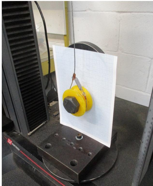
**Figure 6.2:** Modified clevis arrangement to permit visual assessment of the behaviour of the snare over the spool when under load (at the start of the test before any load has been applied).
