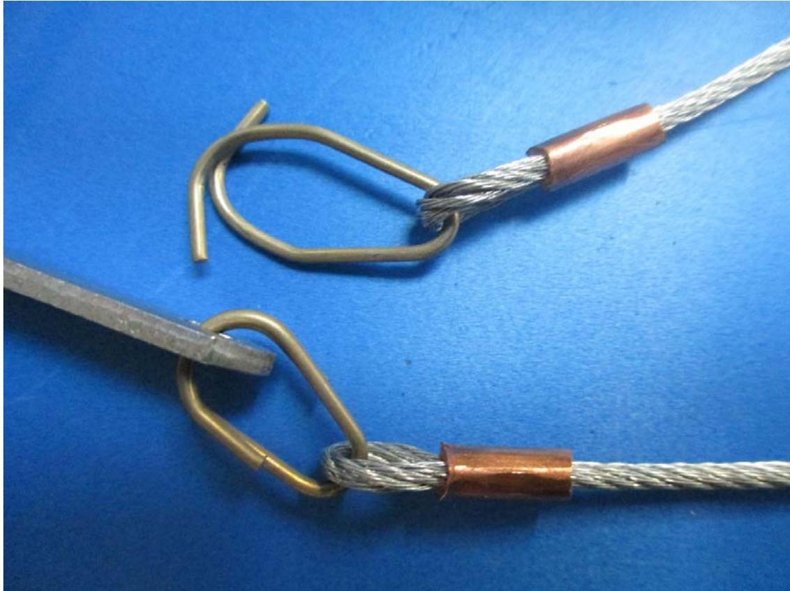
**Figure 5.2:** Appearance of the breakaway clip failures (top) compared with untested clip (bottom).
