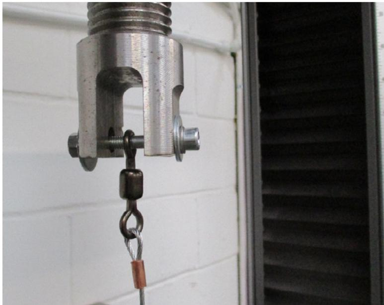
**Figure 3.2:** Ground swivel mounted on the 30 kN load cell by M6 steel bolt.
