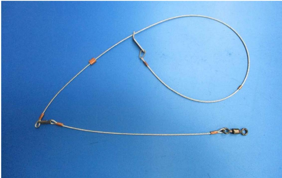
**Figure 2.1:** Overview of example DB type snare supplied for testing.
