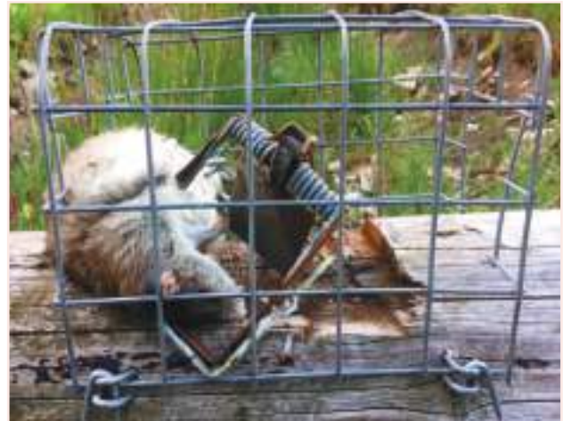
Figure 8. Rat struck by one arm of a Fenn trap, on the thorax. It is a large rat and it is unknown how quickly it died. The wire hoop is only 125 mm long, and the lack of effective excluders meant that any non-target species could have been caught in the trap. Photo: B. Thain.
