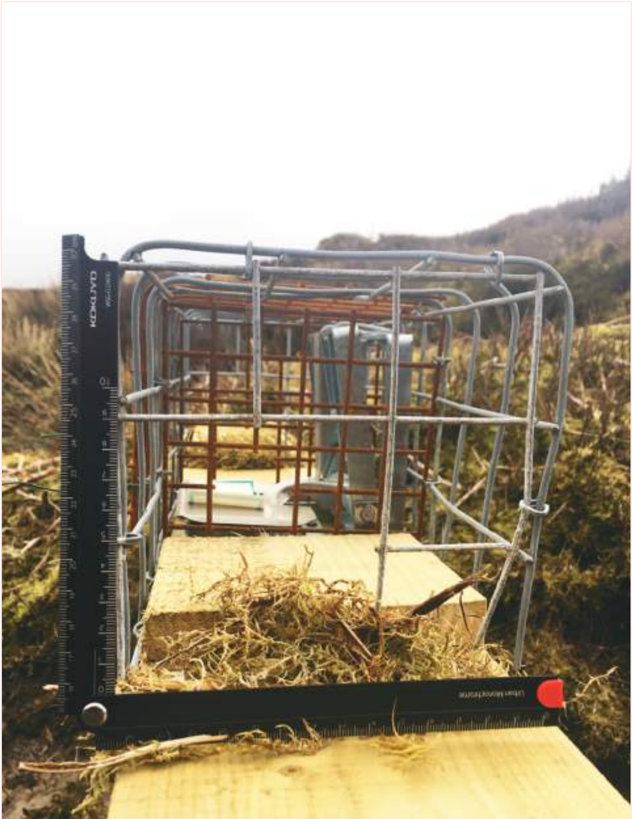
Figure 25. DOC trap set in a poorly restricted wire hoop on a plank across a stream on a grouse moor in Lancashire, 2021. The entrance holes are not offset from the baffles. It is very doubtful whether this trap would exclude birds and protected mammals.
