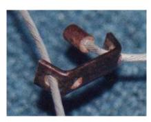
The only way to tell is to take a close look at the metal bracket through which the wire is threaded. This close up view of the bracket on the snare above shows that the wire is threaded through the outermost of the two holes in the bracket. This is what makes the snare self-locking.
