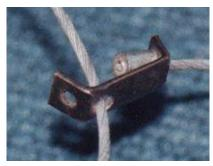
Here is a close up view of the metal bracket on another dualpurpose snare. This time, the wire is threaded through the innermost of the two holes in the bracket. This makes the snare a legal free-running snare.
